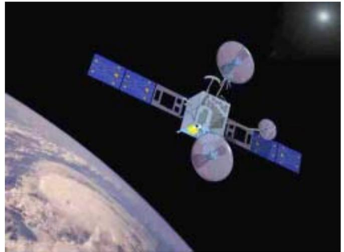
*EO-3, carrying the GIFTS instrument, will be in a geosynchronous orbit for extended monitoring of large regions of our planet and enabling observation of weather patterns at higher resolution than possible with existing geostationary satellites.*
