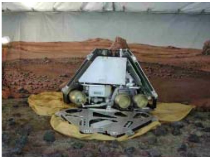
A full-size model of the Mars Exploration Rover with one petal deployed. Photos courtesy of Mojo.
