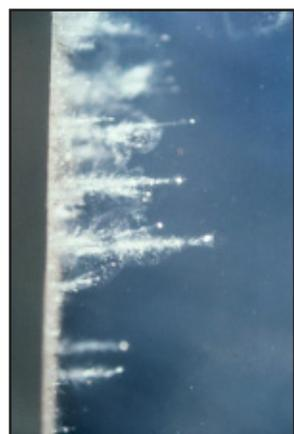
In an experiment on Earth, researchers used a special gun to fire particles into an aerogel. As the particles slowed to a stop, they left carrot-shaped tracks.
